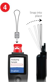
Position collector in an upright position with the oral collection point facing downward
